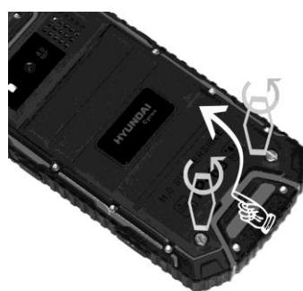
2) Remove the battery if it is inserted in the device.
